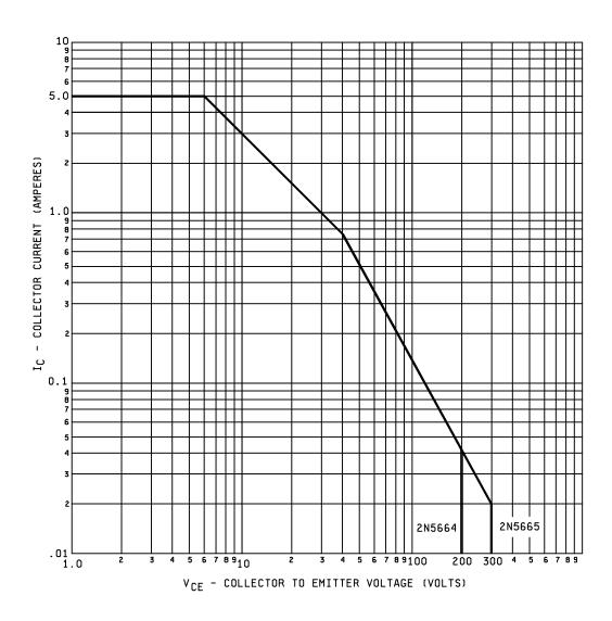
FIGURE 6. Maximum safe operating graph (continuous dc) for types 2N5664 and 2N5665.
