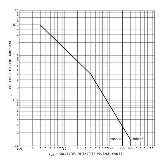
FIGURE 7. Maximum safe operating graph (continuous dc) for types 2N5666, 2N5666S, 2N5667, and 2N5667S.
