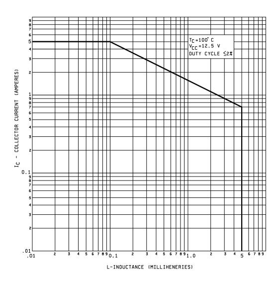
FIGURE 9. Safe operating area for switching between saturation and cutoff (unclamped inductive load).
